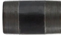
2" DIAMETER DIAMETER BLACK EXTRA HEAVY XXS SEAMLESS Wall Thickness 0.436 - Grade B - Test Pressure 2500 PSI - Thread Length 1.06
