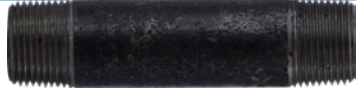
3/4" DIAMETER DIAMETER BLACK EXTRA HEAVY XXS SEAMLESS Wall Thickness 0.308 - Grade B - Test Pressure 1000 PSI - Thread Length 0.79
