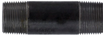
1" DIAMETER DIAMETER BLACK EXTRA HEAVY XXS SEAMLESS Wall Thickness 0.358 - Grade B - Test Pressure 1000 PSI - Thread Length 0.98
