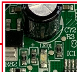
LED1: Drive failure indicator
