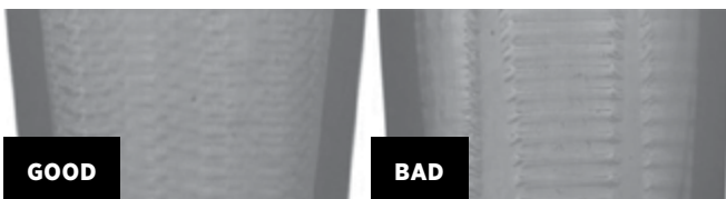
Cut away of PEX piping after proper and improper expansion
