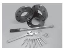
4. The bolts on the plastic flanges should be tightened by pulling down the nuts diametrically opposite each other using a torque wrench. Complete tightening should be accomplished in stages using the final torque values (see table on next page) Recommended Torque. Uniform stress across the flange will eliminate leaky gaskets.
