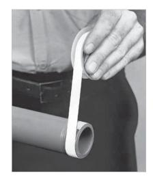
number two thread from the end. The tape should slightly overlap itself going in the same direction as the threads. This will prevent the tape from unraveling when the fitting is tightened on the pipe. Overlapping in the wrong direction and the use of too much tape can affect tolerances between threads. This can generate stress in the wall of female fittings resulting in failure during operations.
