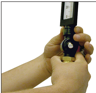
Rotate locking nut by hand.
