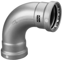
MegaPress FKM is a carbon steel, cold press system designed for use in chilled water, hydronic heating, compressed air, and fire sprinkler applications. MegaPress FKM fittings in sizes from ½" to 4" are offered in configurations including: elbows, couplings, no-stop couplings, reducers, tees, reducing tees, adapters, unions, caps, and flanges.
