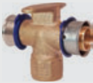
Viega PEX Press Tee Zero Lead - For fire sprinkler systems - Only use with ViegaPEX Ultra tubing Model V5009.1,V5009.51 - Bronze - Press connection, female pipe thread - Mounts to horizontal surfaces Note For use with black ViegaPEX Ultra only. UL listed for NFPA 13D systems Model 2818.2ZL
