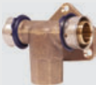
Viega ProPress Tee Zero Lead - For fire sprinkler systems - Only use with ViegaPEX Ultra tubing Model V5009.1,V5009.51 - Bronze - Press connection, female pipe thread - Mounts to vertical surfaces Note For use with black ViegaPEX Ultra only. UL listed for NFPA 13D systems Model 2818.3ZL
