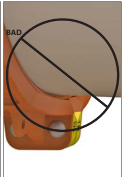
IMPROPER INSTALLATION DUE TO UNEVEN TIGHTENING – COUPLING KEY ON TOP OF PIPE OD
