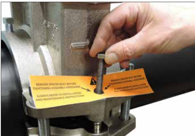
5c. REMOVE ONLY THE SPACER BOLTS: There is one spacer bolt on each bolt pad to maintain spacing between the bolt pads during shipping and assembly. After inserting pipe, remove only the spacer bolts and the attached warning tags before tightening the four nuts in step 6.
