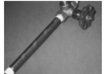
Step 8: Assemble the 1/2" X 6 1/2" (15 X 165 mm) long nipple (Item #6) and the 1/4" pipe plug (Item #7) to the remaining 1/4" NPT three way globe test valve (Item #2) using a suitable teflon tape or pipe dope.
