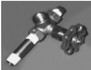
Step 5: Assemble the 1/4" X 2" (6.4 X 50 mm) long nipple (Item #5) and a 1/4" 6.4 mm pipe plug (Item #7) to the 1/4" (6.4 mm) NPT three way globe test valve (Item #2) as shown using suitable pipe dope or teflon tape.
