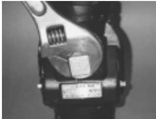
Step 1: Remove 2" (50 mm) NPT pipe plug.
