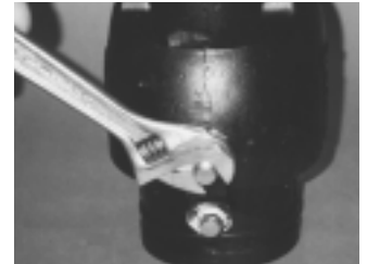
Step 4: Remove both 1/4" (6.4 mm) NPT pipe plugs.
