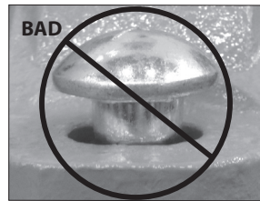
OVAL NECK OF BOLT NOT SEATED PROPERLY
