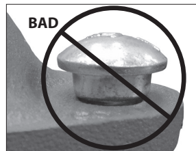
OVAL NECK OF BOLT NOT SEATED PROPERLY
