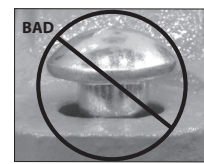
OVAL NECK OF BOLT NOT SEATED PROPERLY
