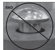
OVAL NECK OF BOLT NOT SEATED PROPERLY
