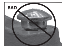
OVAL NECK OF BOLT NOT SEATED PROPERLY
