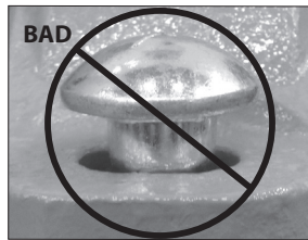
OVAL NECK OF BOLT NOT SEATED PROPERLY
