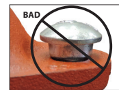
OVAL NECK OF BOLT NOT SEATED PROPERLY
