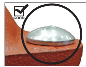
OVAL NECK OF BOLT SEATED PROPERLY OVAL NECK OF BOLT NOT SEATED PROPERLY
