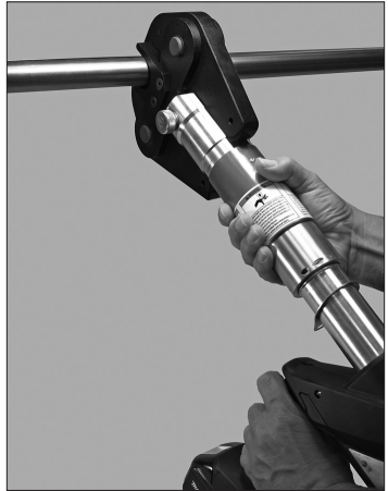
Press Ring/Vic-Press Adapter Jaw Assembly for 1½-inch/48.3-mm and 2-inch/60.3-mm Sizes
