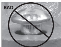
OVAL NECK OF BOLT NOT SEATED PROPERLY
