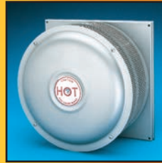
Standard Vent Assembly — Direct Vent Counterflow — accommodates wall thickness from 3/4" (recessed) to 12". Requires 9 1/4" wall opening.
