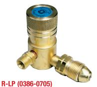
Brass regulator for use with MAP-Pro<sup>™</sup>, Propane and other LPG fuel gas. Adjustable to 60 psi. Fits standard POL valve & 9/16" 18 LH hose nut. Not for use with Acetylene. R-LP-993 Regulator for British 993 Markets, Part No. 0386-0328 Μ
