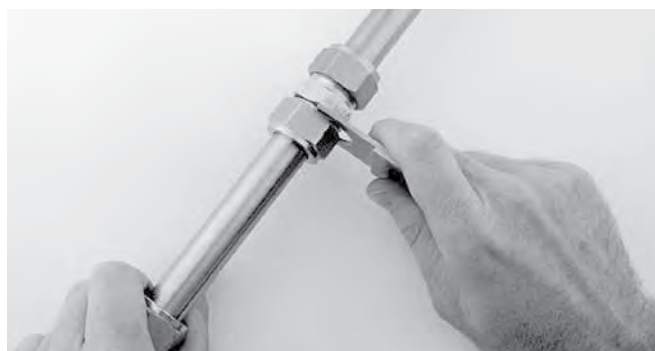
When fitting is properly tightened, gap gage should not fit between nut and shoulder of body.
