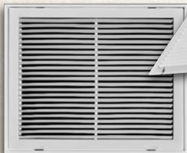
Model 290 Fixed Bar Return Air Filter Grille 3/4" blade separation 60° blade angle from face
