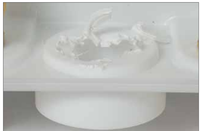
Knockout Problems. Styrene knockouts take extra time, leave a jagged edge and can clog up the drain.
