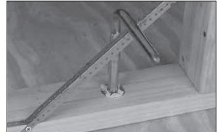
Solder copper tube directly to copper-plated models.
