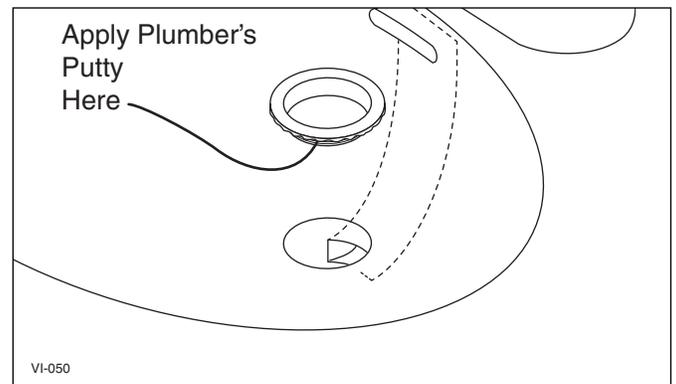
**Note:** When installing the sink ring and tail pipe, use plumber's putty sparingly and do not allow it to contact the plastic overflow assembly under the sink.
