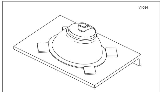
5. Using construction adhesive, fasten plywood strips to countertop surface. For maximum adhesion of plywood strip to countertop, use the manufacturer's recommended curing time.
