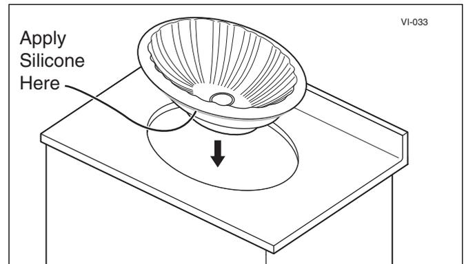
10. If installing for drop-in mount, apply adhesive on the underside of bowl flange and set bowl into opening.
