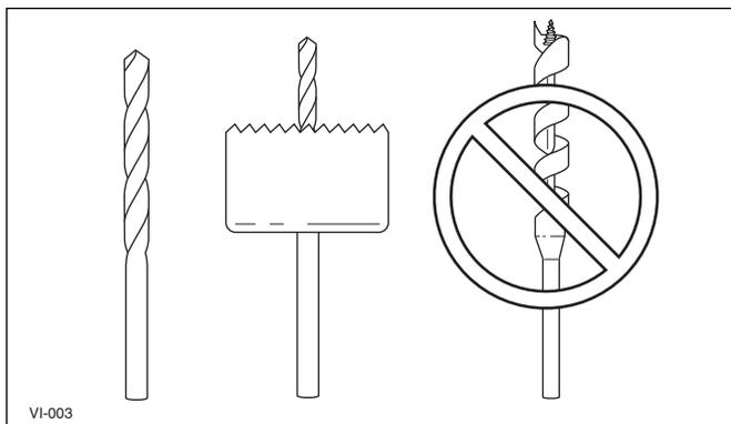
2. Drill fixture hole(s), using the 1/4" pilot hole for a guide, with a 1-3/8" hole saw.
