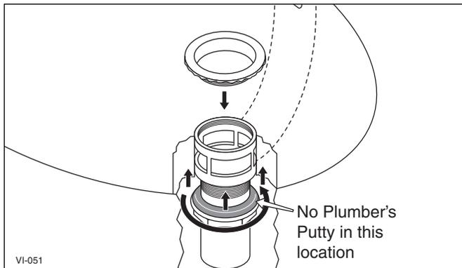
14. Tighten the tail pipe assembly onto the sink
