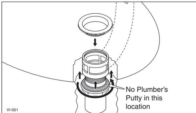
9. Tighten the tail pipe assembly onto the sink.
