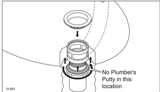
18. Tighten the tail pipe assembly onto the sink
