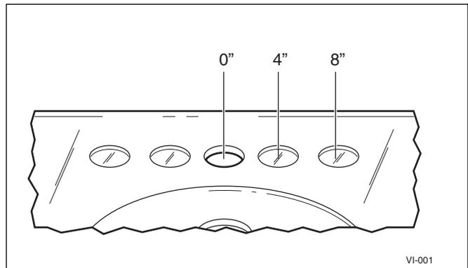
1. If necessary, identify the location of additional holes for the faucet or other accessories and drill a 1/4" pilot hole from the back side of the sink.
