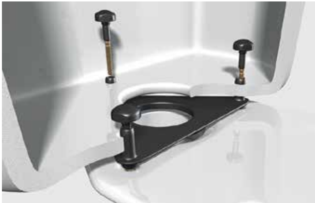
THREE-BOLT INSTALLATION Three preinstalled encapsulated bolts save installation time, provide more leveling adjustment capability, and prevent corrosion.
