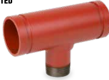
Fig. 65RTT & 66RTT Reducing Tee - Grooved x Male NPT
