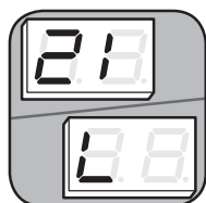
Active Protection – Code 21L – Open low-pressure control
