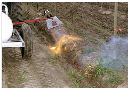
Flaming applies intense heat to weeds and grass causing the cell structure of the plant to be destroyed. You do not have to burn weeds to a crisp.
