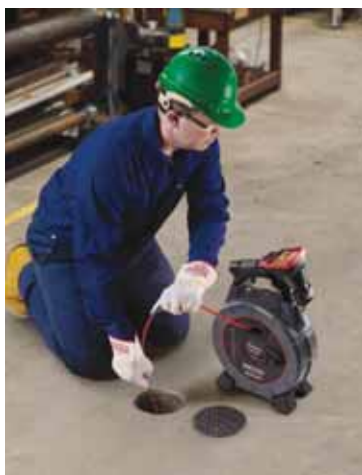
SeeSnake microDrain with micro CA-350 used as a monitor and recording device.
