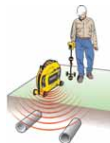
Induce a signal to locate utilities.
