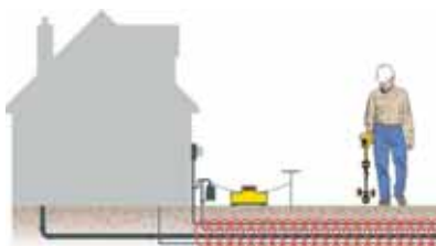
Direct connect to utility lines.
