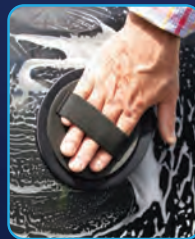
2 Rub RBL Clay Mitt/Disc over area to remove surface contamination
