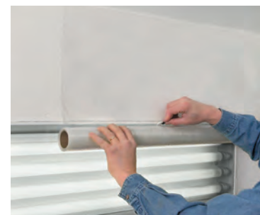
Using a SNIPPET KNIFE or razor blade, cut across film at top edge of lightbox. (Do NOT cover lightbox*.)
