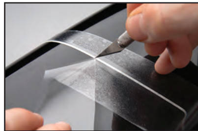
Transparent film improves the accuracy of cutting out sharper details (i.e., cutting the film along the edge of the fine line tape.)
