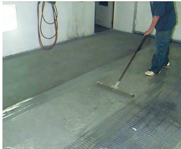
Film can be rinsed off and squeegeed.
