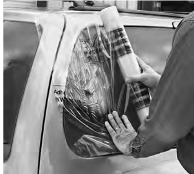
24" width covers side windows in one strip.
