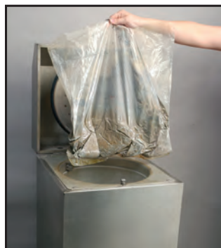
Collected dirty, gummy solvent debris ready for disposal. (In accordance with local regulations.)
