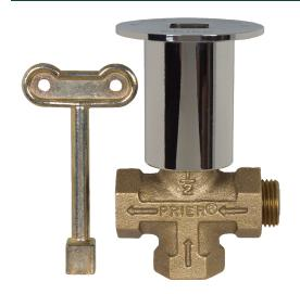
The C-64 Gas Valve is a 3-way design, allowing for installation as a straight or angle valve. This design allows one valve to be used in multiple applications.
