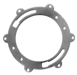
Unique screw tabs attach to wood or concrete. Plastisol coat provides corrosion protection. Slotted for 1/4" or 5/16" closet bolt. Old closet ring does not need to be present. Replaces any and all closet rings.
