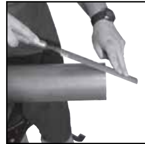
Figure 4: Deburr outside diameter using a half-round file
