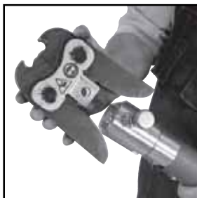
Figure 7: Placement of adapter jaw into the tool
