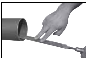
Figure 2: Deburr inside diameter using a half-round file
