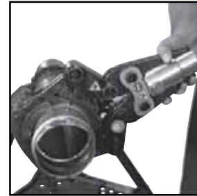
Figure 8: Placement of adapter jaw into pressing chain
