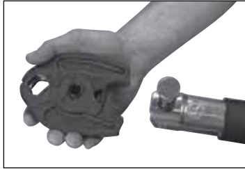
Figure 5 — Inserting the NIBCO® Press System® jaw
