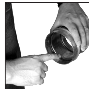
Figure 5: Check for EPDM seal
