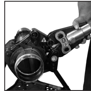
Figure 8: Placement of adapter jaw into pressing chain
