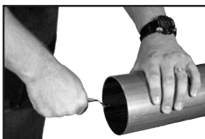
Figure 3: Deburr inside diameter deburring tool
