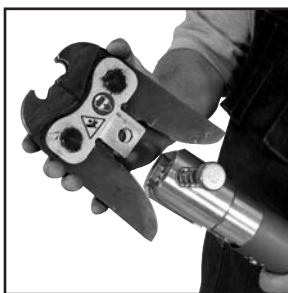
Figure 7: Placement of adapter jaw into the tool
