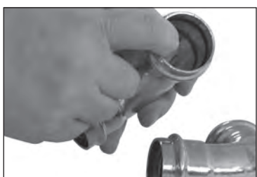
Figure 2 — Check for EPDM Seal
