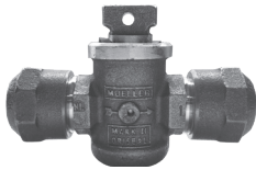
Mueller MARK II ORISEAL Curb Valve Inlet: CTS Kitec Compression Outlet: Mueller 110 Compression for CTS O.D.* tubing Quarter turn check
