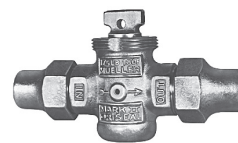
Mueller MARK II ORISEAL Curb Valve Copper flare nut - both ends Quarter turn check, Minneapolis thread top and drain
