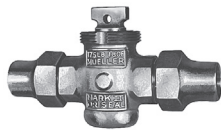
Mueller MARK II ORISEAL Curb Valve Copper flare nut - both ends Quarter turn check and Minneapolis thread top
