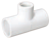
Reducing Tee SLIP x SLIP x FPT
