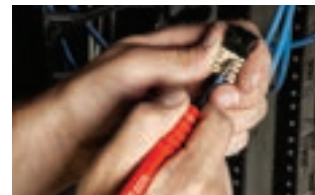
Wire Pick & Hook for Removing Errant Connections
