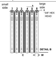
MIFAB's 5"-12" no hub couplings have six sealing bands. Tighten the bands to minimum 80-inch pounds torque, alternatively in the following sequence: 3, 2, 1 - 4, 5, 6
