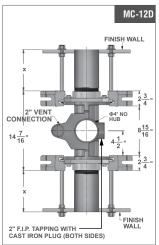
**Note:** 8" tapered thread ABS nipple shipped standard with MC-10 Series carriers. The universal faceplate assembly accepts all nipple variations, rolling thread (-OR), cast iron (-CI) and tapered thread ABS with adjustable horn (-AH).
