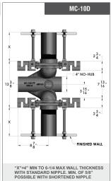
\*MC-10 is tested to support a 500 lb. load with the rear anchor support.
