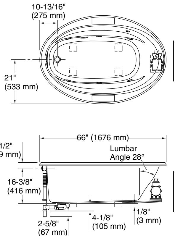
No change in measurements if connected with drain illustrated. (K-37382)
