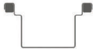
Specify: With Solid Bar Reinforcement
