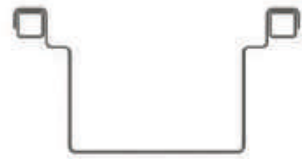
Specify: With Box Section Reinforcement
