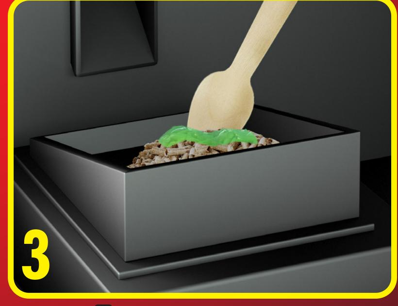
Mix well. Use an old spoon or a rigid tool to stir the pellets. Doing so will ensure the gel is well distributed amongst the pellets, allowing better ignition and combustion.
