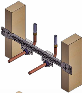
SINK Copper to PEX 1/2" Solution HoldRite ProGuard® #SB3-7312
