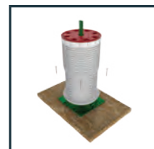
Nail to form deck
