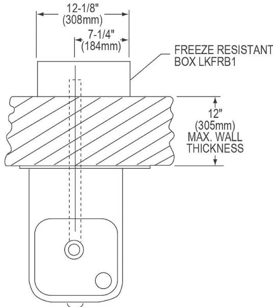
**WARNING:** The freeze-resistant box must be installed on an interior heated wall where the temperature does not drop below 50° F (10° C). The front of the box must have unobstructed air flow. Failure to maintain the interior wall temperature and the inside of the freeze resistant box above 50° F (10° C) can result in damage to the box which could result in unrestricted water flow.
