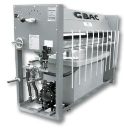
The GBAC applies Duro Dyne WIT or WSA water base adhesive to insulation in preparation for application to sheet metal. It requires 110v service fused for 15 amps. A source of air is required. Specify the direction of work flow when ordering.
